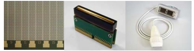
Fig. 1. (a) The cell layout of a CMUT device; (b) a fully-packed CMUT probe head; (c) a fully assembled CMUT probe for ultrasound imaging.
